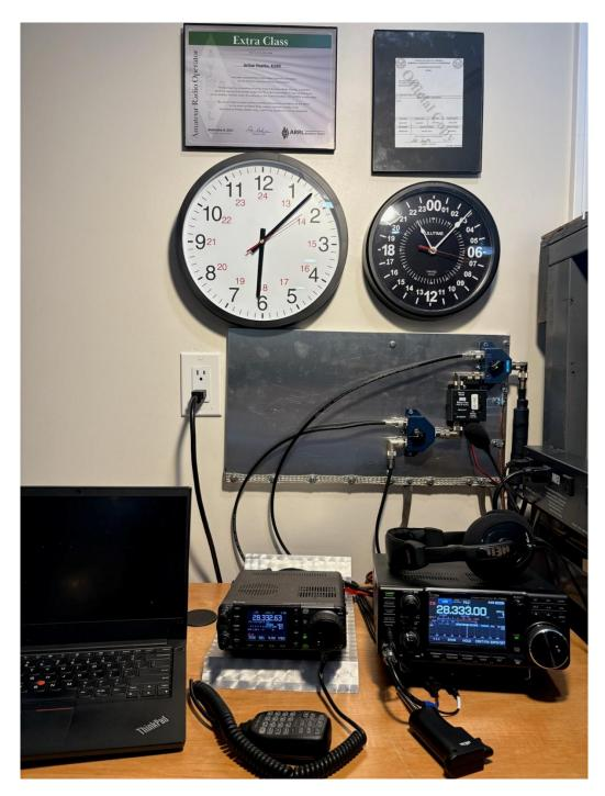
This month, Art, k2IIR was kind enough to send us a photo of his nice shack. The radios shown are an Icom IC-7300 (HF/50 mHz) and an Icom IC-7000 (Predecessor to the IC-7100, HF/VHF/UHF all mode). The main antenna is a ¼ wave (on 160) wire approximately 123 feet long. He also finds the antenna to even be effective on the 2 meter band where it is 20 +/-wavelengths long!
